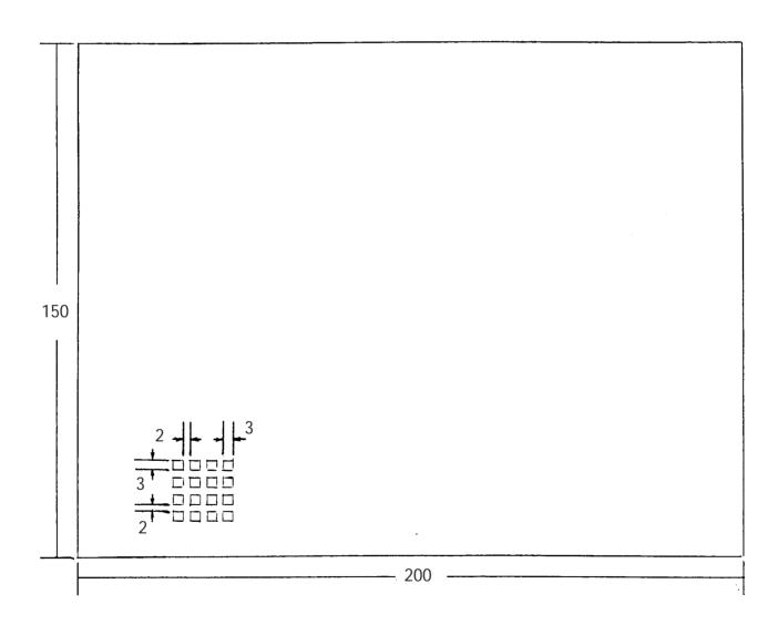
The square holes cover the whole of the sheet, on a 5mm matrix, from the centre line of each hole.
