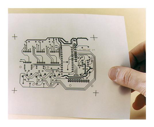
A specially formulated translucent film for the production of high resolution PCB artworks directly from any Laser printer. LaserStar has a 75 micron base with a special coating for high resolution keying and fixing of toner enabling crisp dense artworks to be produced. The film will also accept copier toner enabling usable artworks to be produced from pre-printed originals.
