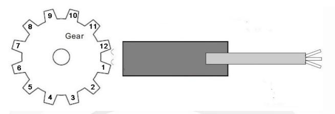
Therefore the scale required is  $1 \div 12 = 0.083$  this is then entered into the scale box which will then mean the scale on the APM can read true RPM
