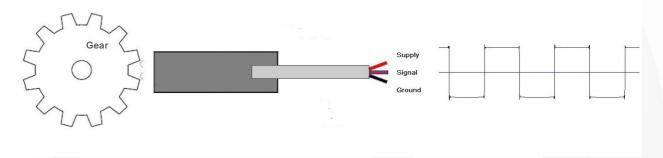
The APM-FREQ detects and measures the frequency of the output from the inductive sensor. The AMP-FREQ maximum frequency is 400Hz therefor consideration must be made when designing the system to ensure that the maximum frequency from the system will not exceed this.
