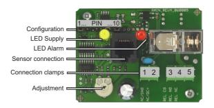
A further probe (special accessories) can be connected to the sensor connection, which can be additionally monitored by the built in electronics.
