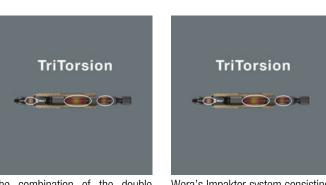
The combination of the double torsion zones in the Impaktor holder and the torsion zone in the Impaktor bit result in the so-called TriTorsion system.
