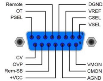
**Attention! Never connect grounds of the analogue interface to minus (negative) output of an external control application (PLC, for example), if that control application is otherwise connected to the neative power supply output (ground loop). Load current may flow over the control leads and damage the device!**
