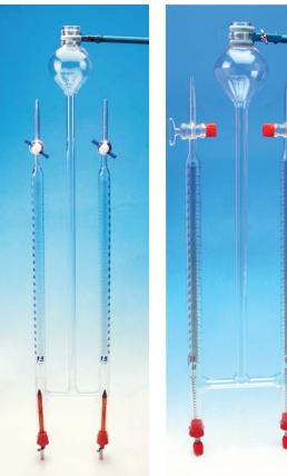
Platinum electrodes mounted in rubber stoppers are used for the electrolysis of acidified water but carbon electrodes must be used for ammonia solutions or hydrochloric acid (or another chloride containing solution).
