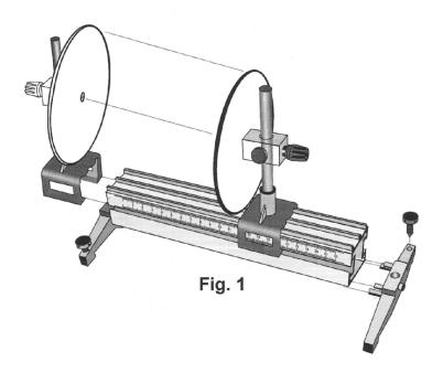
Position the round plate against the plastic pillar & fit with the screw given on the bashed. Position the plate at the same level.
