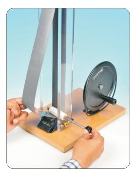
9. Tighten set screw with allen wrench. To ensure set screw aligns with flat rectangle of axle, it may help to turn pulley with one hand while tightening set screw with the other.
