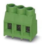
PCB terminal block, nominal current: 32 A, nom. voltage: 630 V, pitch: 7.62 mm, number of positions: 3, connection method: Screw connection with tension sleeve, mounting: Wave soldering, conductor/PCB connection direction: 0 °, color: green. The article can be aligned to create different nos. of positions!
