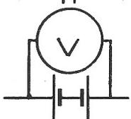
Turn one of the cells the wrong way round. Is there any driving force available when the cells are connected this way?
