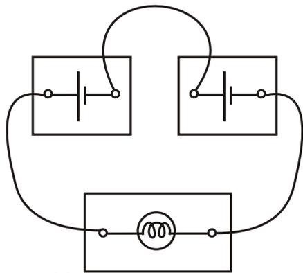
For example, in experiment 2 you set up a circuit which had 2 cells connected to one bulb like this:-
