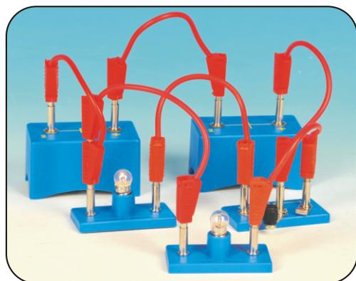
Set up the circuit shown here with two changeover switches. This circuit is unusual in that two switches are used to control only one light bulb.
