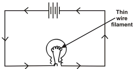
In this simple circuit the electricity has to flow through the bulb. If you look at a bulb closely you will see that the electricity passes through an extremely thin wire called a FILAMENT. As you have already learned, very thin wires have a very high resistance than thick wires. So this resistance will keep the electrical current down to a safe value.
