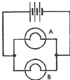
Use two switches in this circuit so that when one switch is pressed, lamp A lights up and when the other switch is pressed, lamp B lights up.
