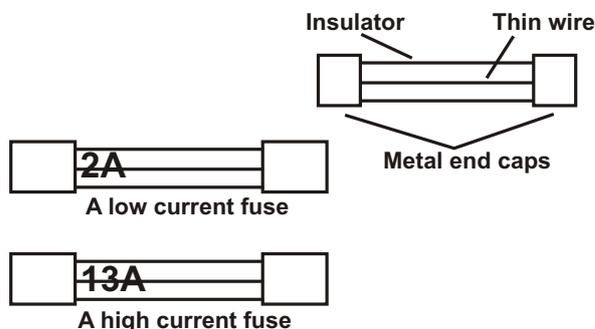
Equipment such as electrical heaters take a large current so are fitted with thick wire fuses, e.g. "13 amp", but low current equipment such as lights or a television set need a thinner wire fuse, e.g. "2 amp".
