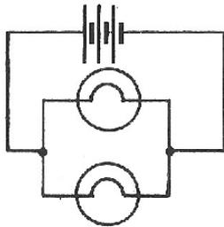
Place a switch so that one lamp stays on all the time but the other only lights when the switch is pressed.
