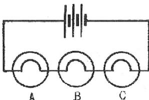
Use two switches in this circuit so that when one switch is pressed ALL the lamps light but, if the other switch is pressed only lamp C lights up.
