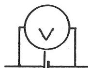
First of all, try connecting a voltmeter across a single cell as shown here. Note the reading in volts.
