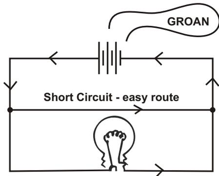
If we add an extra lead to SHORT CIRCUIT the bulb, the electricity will take the easy route round the circuit. So instead of flowing through the high resistance filament, it will go through the low resistance short circuit. Because the resistance is very low, the current will be very high. If the circuit is left on, the battery will be run down very quickly.
