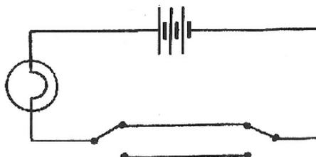
This type of light switching circuit is very common in houses. Try moving each switch in turn to find out what special properties they have.
