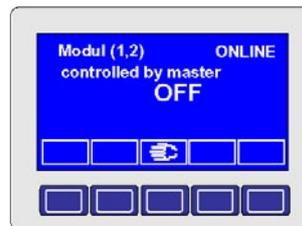
Example: the slave is online and the power output of the system is in standby (switched off). The (1,2) shows that this slave is directly connected to the master in parallel (2).
