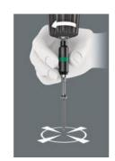
The free-turning sleeve allows screw steadying at the start of the screwdriving process. This makes it easier to apply the tool to the screw and prevents slipping. It can also be used as a short extension for 1/4" applications e.g. in combination with the Wera Zyklop Ratchets.
