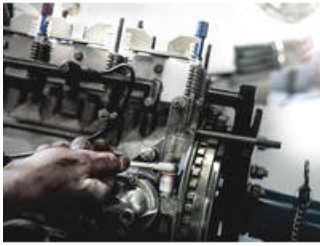
Nutsetter for hexagon head screws
