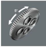
The reversible ratchet with 72 finepitched teeth has a low return angle of only 5°. This short stroke allows fast and precise work in all types of installation.
