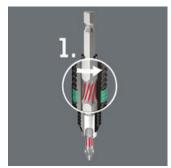
The effectiveness of the BiTorsion system comes from a combination of two shock-absorbing spring elements. Both bits as well as holders have a cushioning torsion zone that diverts the kinetic energy away from the drive tip during peak loads.
