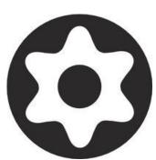
TORX® tools with a borehole prevent the unauthorised unfastening of safety screws. The screws contain a pin that protrudes into the drive profile so that "normal" TORX® tools cannot be used. This pin fits into the borehole of TORX® BO tools allowing safety screws to be unfastened.
