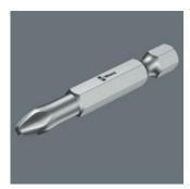
TZ-Bits are tough bits with a torsion zone. Torsion bits absorb the damaging peak torque loads in the torsion zone. This prevents premature wear and enhances the service life of the bits.
