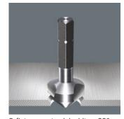
3-flute countersink bits, 90° • Application: Deburring, chamfering and countersinking • ½" drive suitable for holders as per DIN 3126-D 6.3 (ISO 1173) • Hexagon shaft for very high torque transfer • HSS = high speed steel • Finely adjusted material elasticity for long service life • 3 tips • Excellent centring properties • Straightforward cutting • Perfect chip removal • Low jamming risk • Precise return control • High corrosion protection
