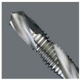
Combination drill bits Application: Core-hole drilling, tapping and deburring in one operation • 1/4" drive suitable for holders as per DIN 3126-D 6.3 (ISO 1173) • Hexagon shaft for very high torque transfer • HSS = high speed steel • Finely adjusted material elasticity for long service life • Excellent centring properties • Straightforward cutting • Perfect chip removal • Low jamming risk Precise return control
