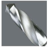
Twist drill bits — for metal applications • 1/4" drive suitable for holders as per DIN 3126-D 6.3 (ISO 1173) • Hexagon shaft for very high torque transfer • HSS = high speed steel with cone point • Finely adjusted material elasticity for long service life • Excellent concentricity • Tough-absorbing tempered bits for particularly long service life
