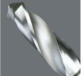
Twist drill bits - for wood applications • 1/4" drive suitable for holders as per DIN 3126-D 6.3 (ISO 1173) • Hexagon shaft for very high torque transfer  $\bullet$  HSS = high speed steel • Finely adjusted material elasticity for long service life • Excellent concentricity • Tough-absorbing tempered bits for particularly long service life
