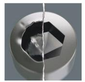
Hexagon screws can endure a problem because the contact surfaces delivering the power from conventional tool, transferred to the screw via very surface areas. consequence: the screw can become damaged (rounding out). Hex-Plus tools have a greater contact surface that prevents this from happening! At the same time, as much as 20 % more torque can be applied. Good to know: Hex-Plus tools fit into every standard hexagon socket screw!
