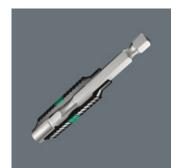
BiTorsion holders from Wera have a torsion spring design that absorbs smaller peak loads during screwdriving. The combined use with BiTorsion bits with their torsion zone distinctly extends the service life of the tool. Conveniently, BiTorsion holders from Wera can also be used with conventional bits.
