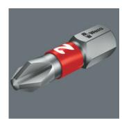
BiTorsion bits are absolutely premium products. They have a softer BiTorsion zone which reduces the hardness of the shaft by about 20 % in comparison to the drive tip. This means that the peak loads that cause bit breakage and premature wear are absorbed in this zone — something which enhances the service life of the bits.
