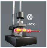
Impact strength tested at  $-40^{\circ}$ C, guaranteeing safety even under extreme conditions.
