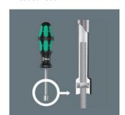
A screwdriver with a hollow shaft is needed whenever there are screwdriving jobs involving threaded rods i.e. the threaded rod through the nut can slip into the hollow shaft of the screwdriver.
