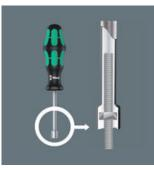
A screwdriver with a hollow shaft is needed whenever there are screwdriving jobs involving threaded rods i.e. the threaded rod through the nut can slip into the hollow shaft of the screwdriver.
