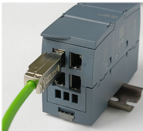
Figure 4-7 Inserting the IE FC RJ-45 Plug 180
