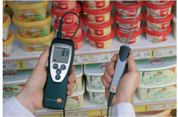
Inspecting the temperature of a refrigerated counter
