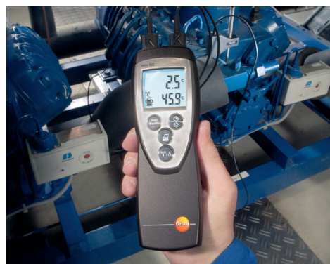
Simultaneous measurement of overheating and undercooling in refrigeration plants
