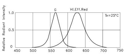
wavelength  $\times$  (nm) RELATIVE INTENSITY Vs. WAVELENGTH
