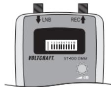
The sat finder can quickly and simply set the satellite system to the best reception level. The sat finder is dragged into the reception line between satellite receiver and receiver unit (e.g. LNB) for this.
