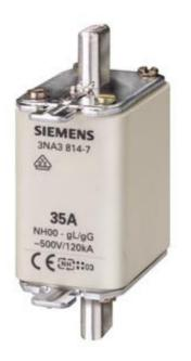
LV HRC FUSE LINK GL/GG WITH NON-INSULATED GRIP LUGS WITH FRONT INDICATOR SIZE 00, 35A, AC 500V/DC 250V
