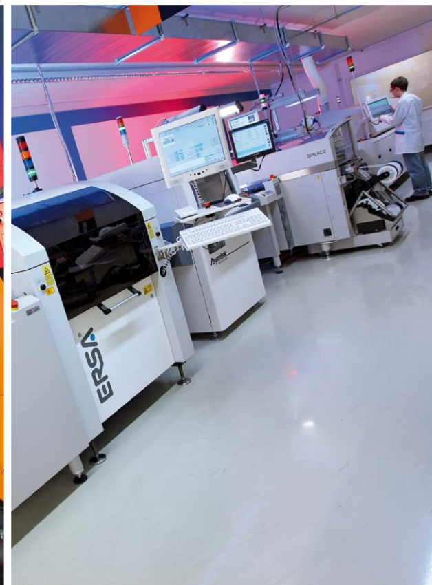
State-of-the-art production lines: SMD printed circuit board manufacturing
