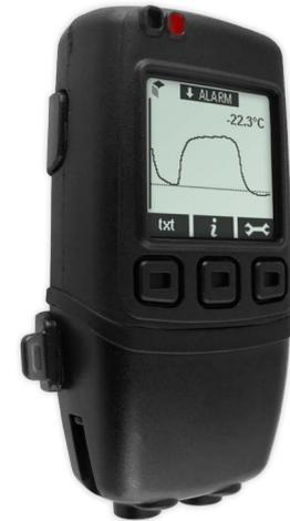
This standalone USB data logger measures and stores over 250,000 temperature readings from two high accuracy thermistor probes over a -40 to +125 °C (-40 to +257 °C) range at a resolution of 0.1°C.
