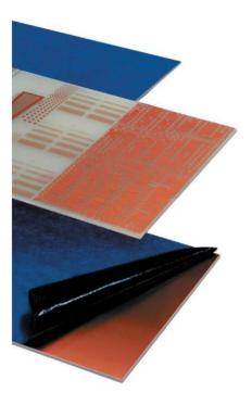
FR4 single and double sided PCB laminated coated with a dip coated high quality positive working Photoresist. Panels are protected by a light proof removable blue film which allows them to be guillotined without the risk of fracturing the photoresist.
