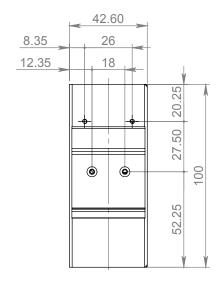
Figure 4. QUARTZ Series - molex connector
