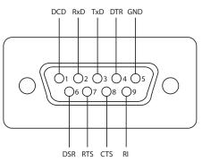
Figure 14. RJ45-DB9 cable
