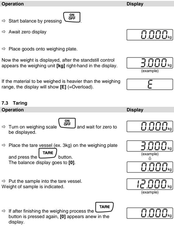
The taring process can be repeated any number of times, e.g. when adding several components for a mixture (adding).
