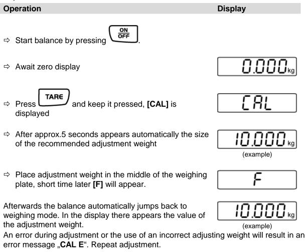
Keep the adjustment close to the balance. Daily control of the weighing exactness is recommended for quality-relevant applications.
