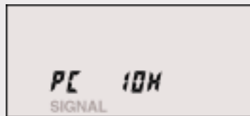
Figure 4. 10 Base-T signal detected, wired to PC.
