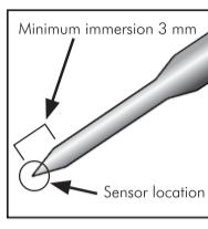
Apply the tip of the probe to the substance, medium or surface to be measured. The sensor is located at the tip of the probe, therefore the minimum depth insertion should be 3 mm.
