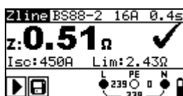
Figure 5.33: Examples of line impedance measurement result
