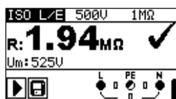
Figure 5.7: Example of insulation resistance measurement result
