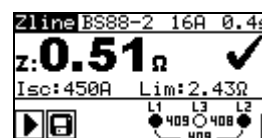
Figure 5.33: Examples of line impedance measurement result
