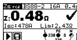
Figure 5.29: Examples of loop impedance measurement result
