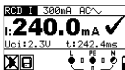
Figure 5.24: Trip-out current measurement result example
