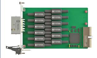
Our Series 67 relays mounted on a 3U PXI 12-Way High Voltage Multiplexer Module, illustrates interesting stacking possibilities.
