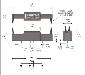
**Important:** Where the optional internal diode is fitted, the correct coil polarity must be observed, as shown by the + symbol on the schematics.
