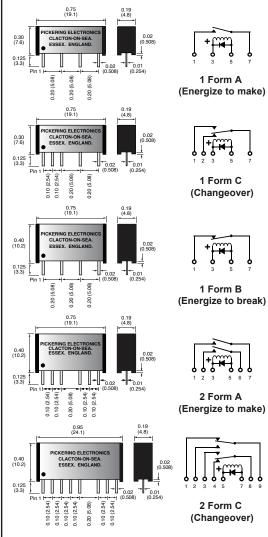
Important: Where the optional internal diode is fitted or for all Form B types, the correct coil polarity must be observed, as shown by the + symbol on the schematics.
