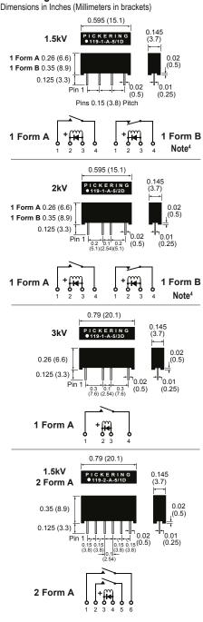
Important: Where the optional internal diode is fitted or for all Form B types, the correct coil polarity must be observed, as shown by the + symbol on the schematics
