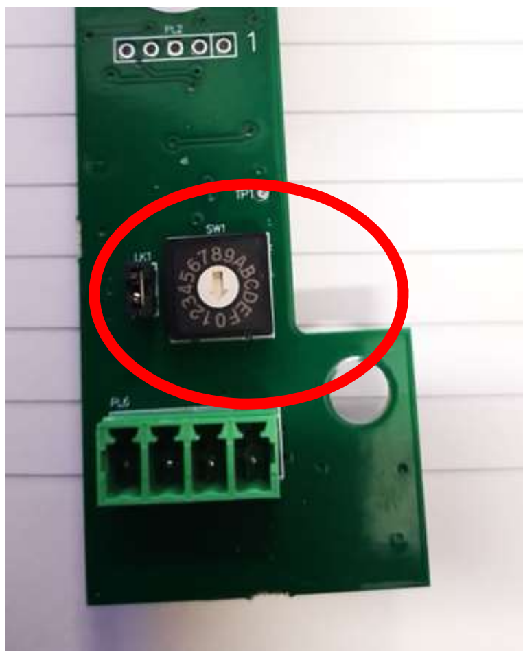
FIGURE 1 - ROTARY SWITCH TO SELECT MAXIMUM CURRENT RATING
