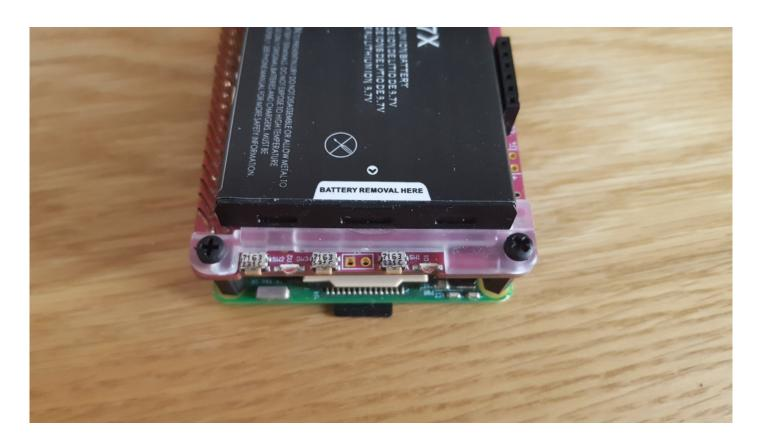
**Step 4** - Unscrew the battery terminals on the PiJuice and insert the wires into the following slots:
