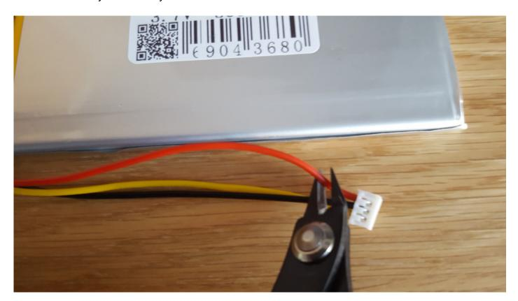
**Step 2** - Carefully cut off approximately 10mm of the outer plastic to expose the bare wires on each wire. Be careful not to cut through the wire. Once the wires are exposed, twist the strands together.
