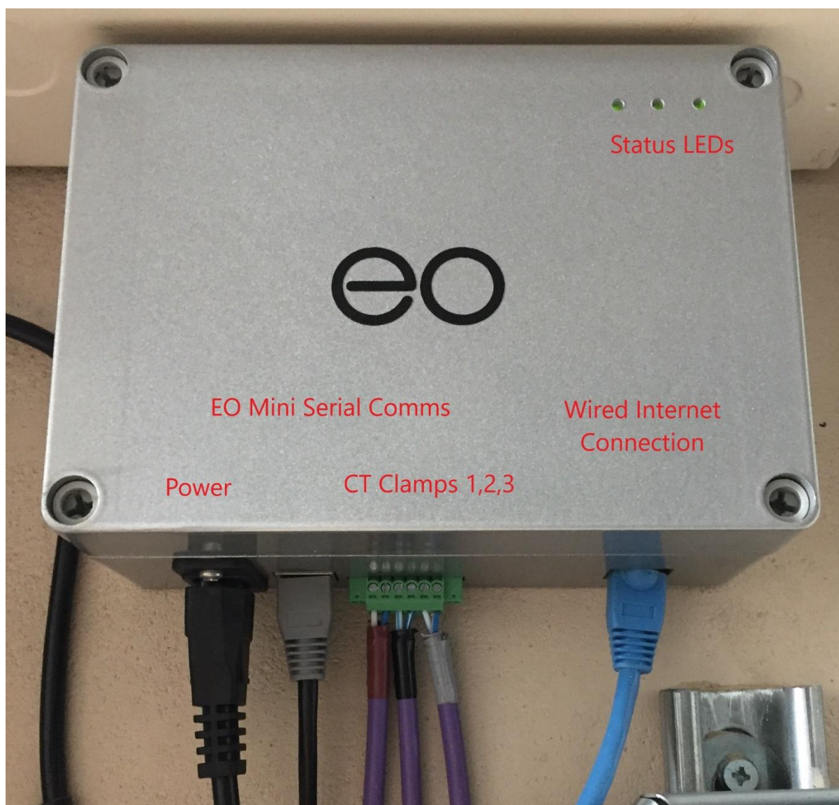
Figure 3 - EO Hub connections
