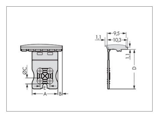
Printview: eCOM pluggable PCB connector with straight solder pins; with gripping plate; 6-pole; Pin spacing 3.5 mm / 0.138 in - Item No.: 2091-1156
