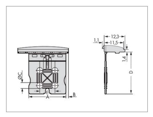
Printview: eCOM pluggable PCB connector with straight solder pins; with gripping plate; 2-pole; Pin spacing 5 mm / 0.197 in - Item No.: 2092-1152
