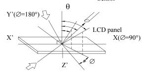
Light (when transmitted )  $Y(\varnothing=0^{\circ})$   $(\theta=90^{\circ})$
